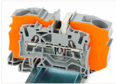
Step-down jumper (2016-499) commons 16/10 mm 2 (16/8 AWG) terminal blocks (2016/2010 Series) with 10/6/4/2.5 mm 2 (8/10/12/14 AWG) terminal blocks (2010/2006/2004/2002 Series).
