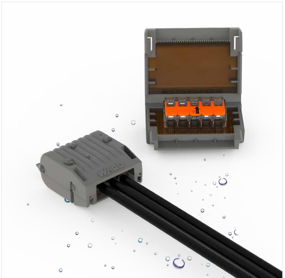
Re-accessible: Open the Yellowox, remove the gel, open the connector and rewire with new components.
