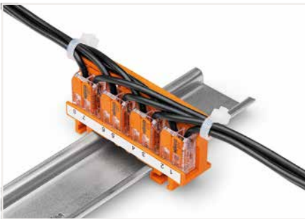
Strain relief via cable ties on the mounting carrier (transverse to the connectors' wiring direction) – clamping units labeled via marking strips (210-334)
