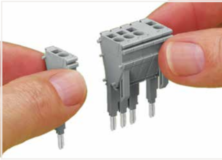
Snapping tap-off and spacer modules together to assemble a multipole tap-off module (max. 10 poles).
