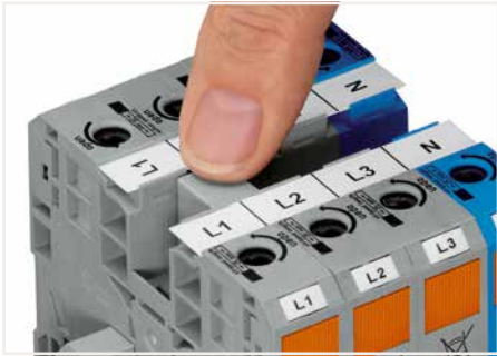
Commoning adjacent terminal blocks using a centrally positioned push-in jumper.
