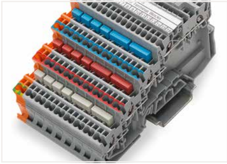
Commoning (potential level): Continuous commoning in the potential levels via push-in type jumper bars for even pole numbers (2000 Series)
