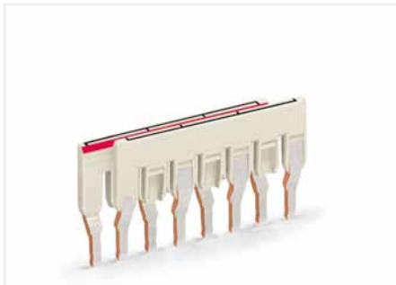
Staggering jumpers in a single jumper slot. Custom staggered jumpers can be created, e.g., for bridging over a terminal block with a different potential. Make sure that only one contact lug is in contact with the terminal block. The contact lugs of the customized staggered jumpers contact the terminal blocks via the gaps created in the second jumper. Insert and press the ready-made jumper assembly into the jumper slot until it hits backstop.
