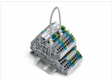
Push down the wire jumper until fully inserted. Lift the jumper with an operating tool for rewiring.
