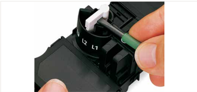
Lift jumper out of delivery position (L2) using a screwdriver and move it into the desired position.
