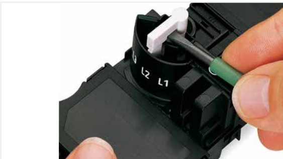
Lift jumper out of delivery position (L2) using a screwdriver and move it into the desired position.
